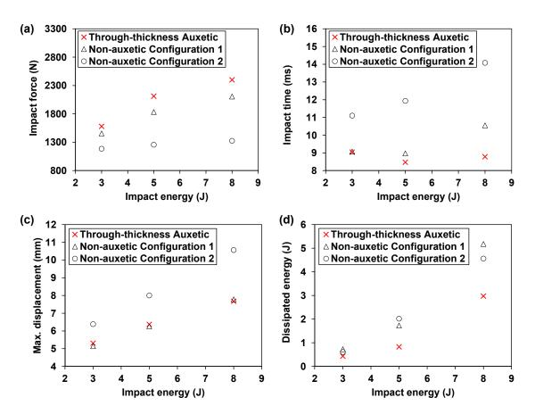
**Figure 6.** Effect of the through-thickness negative Poisson's ratio on the global impact response: comparison between the auxetic and corresponding non-auxetic CFRP composite laminates: (a) impact load, (b) impact time, (c) maximum displacement, and (d) dissipated energy.
