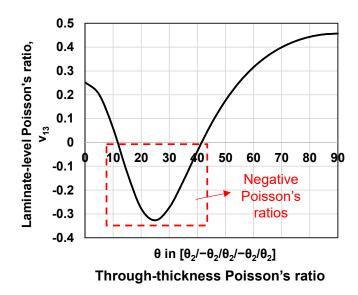
**Figure 2.** Predicted layups to produce laminate-level through-thickness negative Poisson's ratios in IM7/977-3 CFRP composite laminates with a layup of  $[\theta_2/-\theta_2/\theta_2/-\theta_2/\theta_2]$  as the ply angle,  $\theta$ , changes from 0 to 90 degrees.
