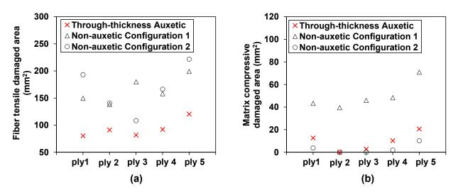
**Figure 12.** Effect of the through-thickness negative Poisson's ratio on the fiber tensile damage and matrix compressive damage: comparison of the predicted damage areas in each ply of the auxetic laminate and the corresponding non-auxetic CFRP composite laminates at an impact energy of 8 J: (**a**) fiber tensile damaged area and (**b**) matrix compressive damaged area.
