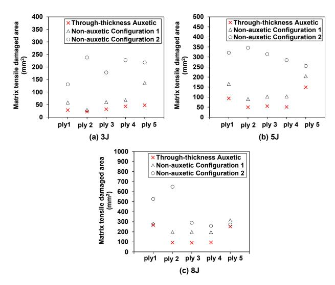
**Figure 10.** Effect of the through-thickness negative Poisson's ratio on the matrix tensile damage: comparison of the predicted damage area in each ply of the auxetic and non-auxetic CFRP composite laminates at: (**a**) 3 J, (**b**) 5 J, and (**c**) 8 J.
