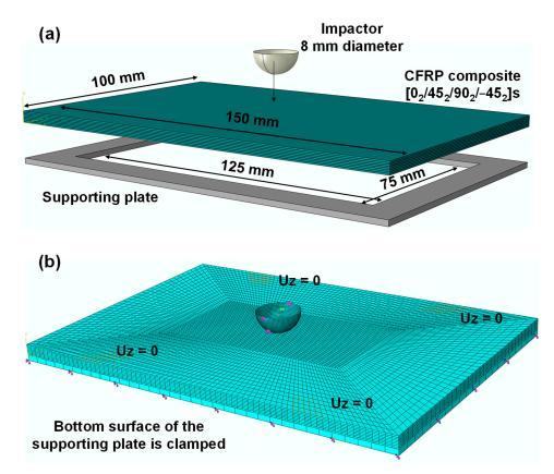
**Figure 3.** Verification of the low velocity impact model using a benchmark simulation problem for a CFRP composite laminate under an impact energy of 25 J: (a) problem setup and (b) mesh and boundary conditions used in the finite element analysis. Note: the x direction represents the longitudinal direction or direction 1, y direction represents the transverse direction or direction 2, and z direction represents the through-thickness direction or direction 3 in the laminate coordinate system.
